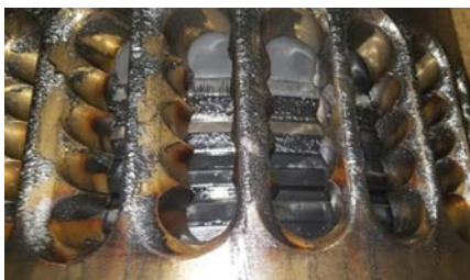
Severely damaged pistons
