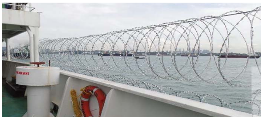
Vessel hardening plan, rigging double layer barbed wires
